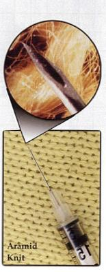
Magnified view of standard cut-resistant glove shows how gaps between aramid fibers can't stop punctures, letting fine penetrators like needles, glass fragments, and metal shards slip past.
